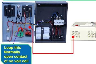
Take a new wire and connect one end to the red-Step 2 Colored push button terminals and the other end to the C-out of the SWAP, as shown in the image below.
